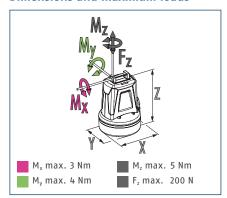
The indicated moments and forces are statical values, apply for each base jaw and should not appear simultaneously. Loads may additionally occur to the moment produced by the gripping force itself.
