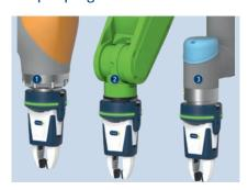
The standard Co-act gripper EGP-C is available for a wide range of collaborative robots (cobots) from a variety of manufacturers including KUKA, Universal Robots and FANUC. The gripper has been pre-configured in a way that it can be mounted directly electrically and mechanically onto the cobots. Depending on the manufacturer, different versions are also available depending on the flange version.
