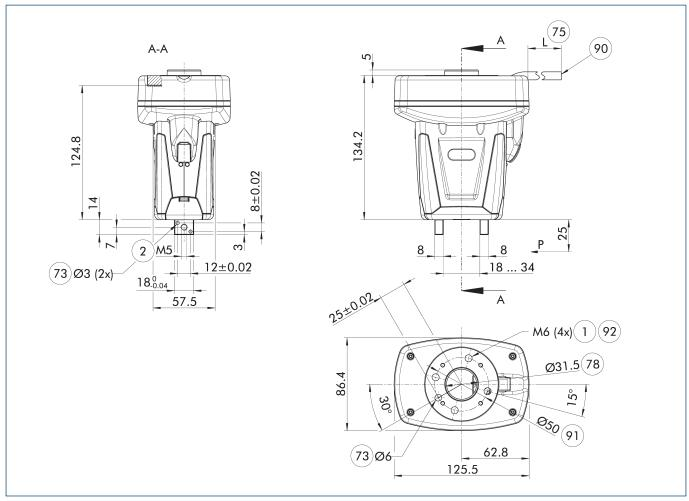
The drawing shows the basic version of the gripper with open jaws.
