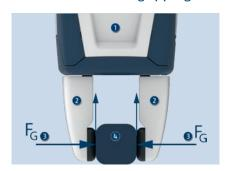
The "gripping force" specification in the catalog refers to the arithmetic sum o the forces acting on each jaw individually at distance P (see illustration). For evaluation of the biomechanical limit values in accordance with ISO/TS 15066, only the gripping force acting on each gripper jaw must be used. Furthermore, the information in the operating manual is referred to.
