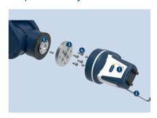
The Co-act EGP-C gripper was developed for simple assembly on collaborative robots (cobots). During assembly, the enclosed adapter plate has to be fastened with the supplied fastening material to the flange of the cobot. Subsequently, the gripper can be fastened with the enclosed hexagon socket wrench to the adapter flange. Finally, the electric connection (not version KETI) must be established.
